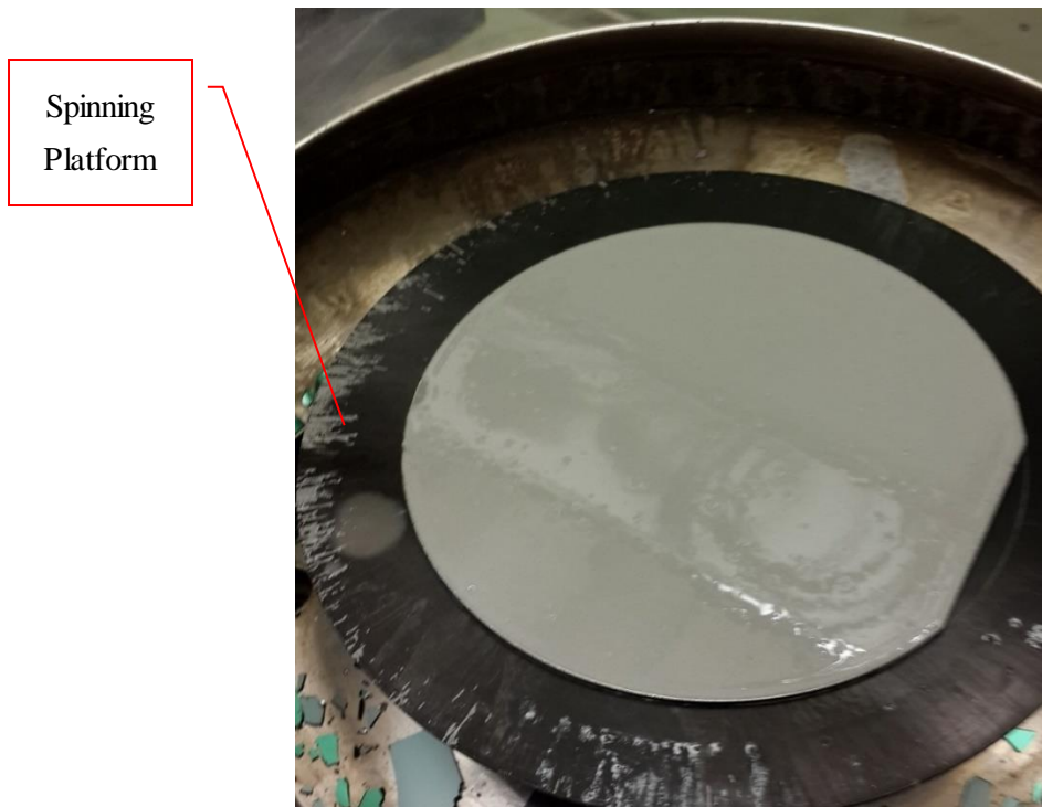
Figure 39 Spin Coating Al Paste: Early Trial. Coated Wafer on Spinning Stage/Platform
