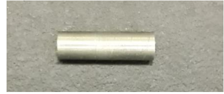
Figure 24 Cylindrical Samples: Extrudate machined into these small cylinders
