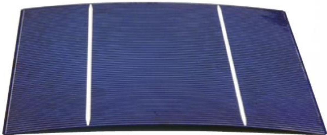
Figure 6 A 160 \mu\text{m} bowed thick solar cell. Figure adopted from Bunkenburg et al, "Enabling thin wafers for today's high efficiency silicon solar cells"
