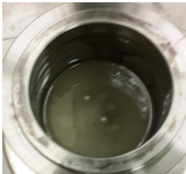
Figure 34 The Organic Vehicle (OV) inside the milling container
