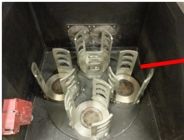
Figure 16 Stainless Steel container holders (Left) in Planetary Ball Milling Machine (Right)
