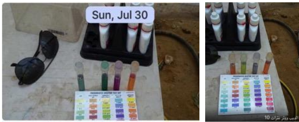
Figure 68: Showing IAVS water test results on the left with Ammonia = 4 vs. Ammonia in DWC = 0.5 on the right (on July 30th, 2017)
