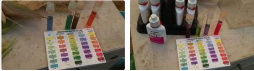
Figure 71: Showing IAVS water test results on the left with Ammonia = higher than 4 (4 – 8) vs. Ammonia in DWC = 0.25 on the right (on July 30th, 2017).
