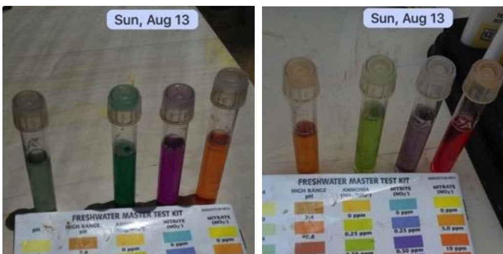
Figure 70: Showing IAVS water test results on the left with Ammonia = 4 vs. Ammonia in DWC = 0.5 on the right (on August 13th, 2017).
