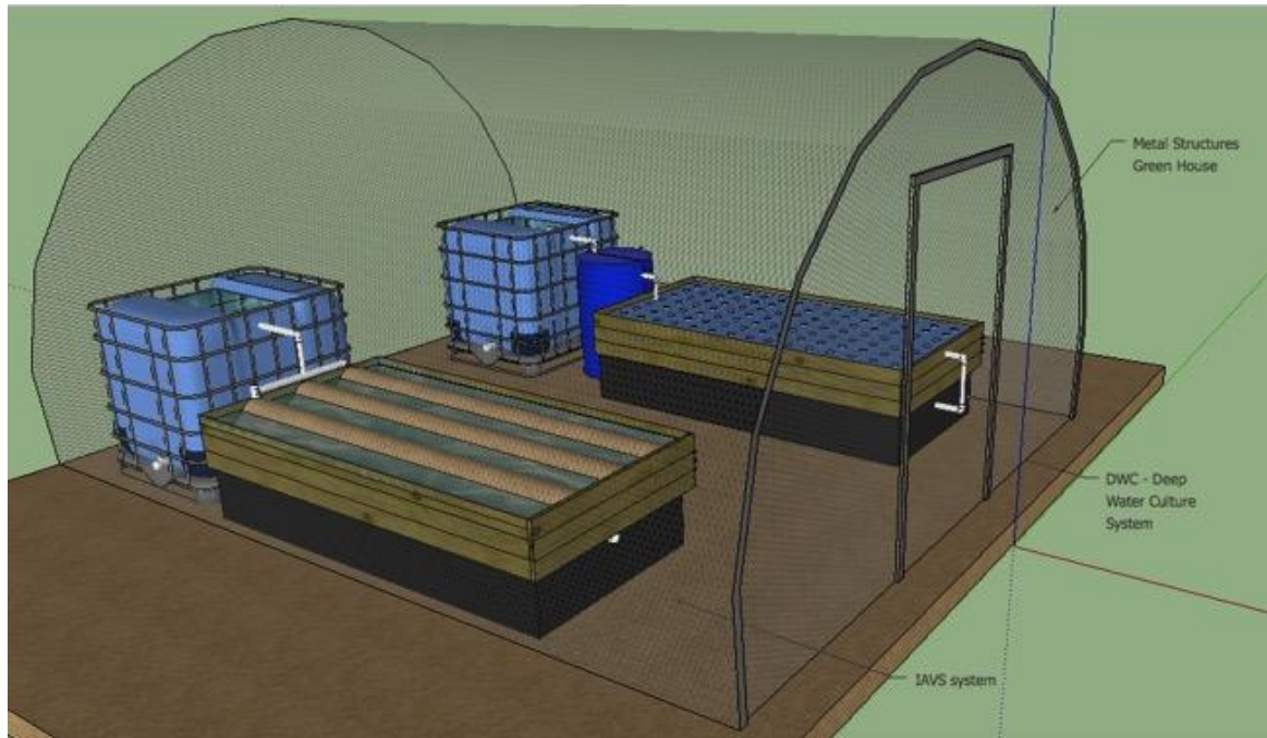
Figure 18: Lab scale of the DWC and IAVS used in the UAC experiment.
