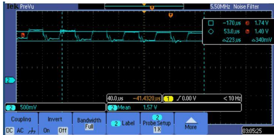
Figure 4.15. Voltage on flying capacitor C1 with cursors.
