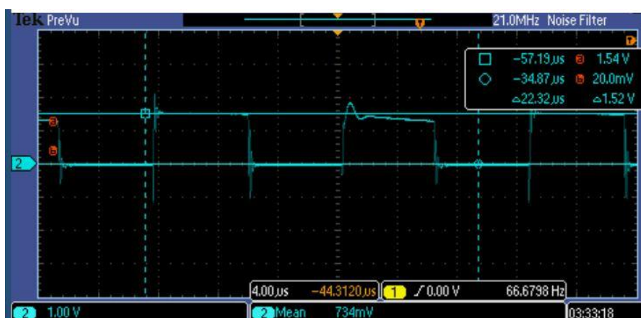
Figure 4.25. Voltage at the inductor of a test 3-Level converter in the first operation region at 50% duty cycle.
