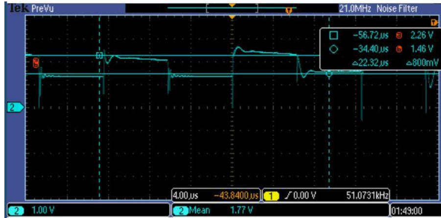
Figure 4.6. Voltage at the Inductor ( V_x ) for the 0.5-0.75V_{in} operation region with 50% duty cycle with cursors.
