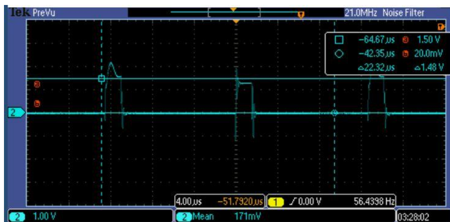
Figure 4.24. Voltage at the inductor of a test 3-Level converter in the first operation region at 25% duty cycle with cursors.
