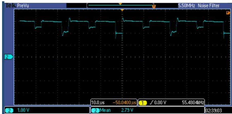
Figure 4.13. Voltage at the Inductor ( V_x ) for the 0.75-V_{in} operation region with 75% duty cycle.
