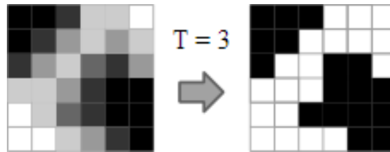
Figure 4-13: Result of Otsu Thresholding at threshold value 3 [38]
