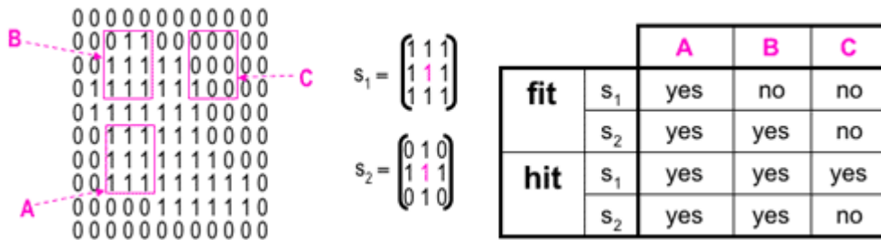
Figure B.2: Fitting and hitting of a binary image with structuring elements s_1 and s_2 . [40]
