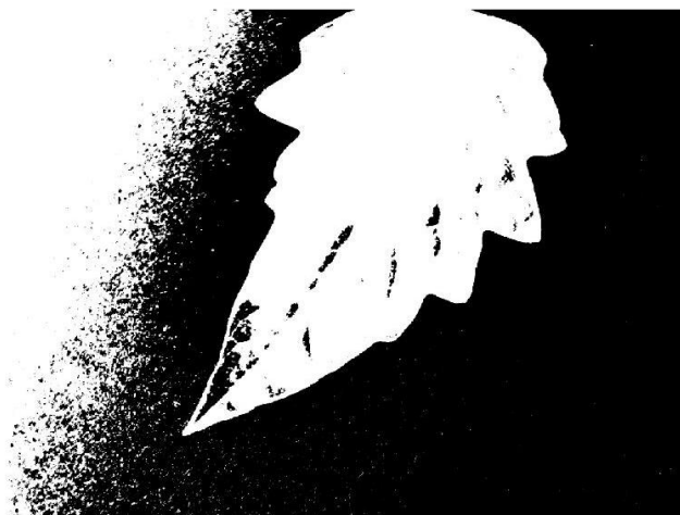
Figure 4-15: iPhone leaf Otsu threshold background segmentation
