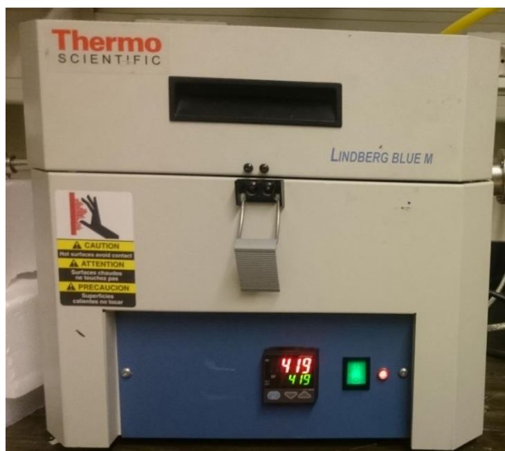
Figure 3.2: Lindberg/Blue M™ Tube furnace, Thermo scientific, used in samples annealing.
