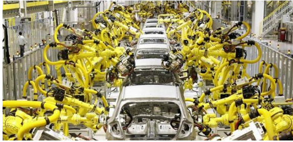
Figure 1.7: Car assembled by robots [4].
