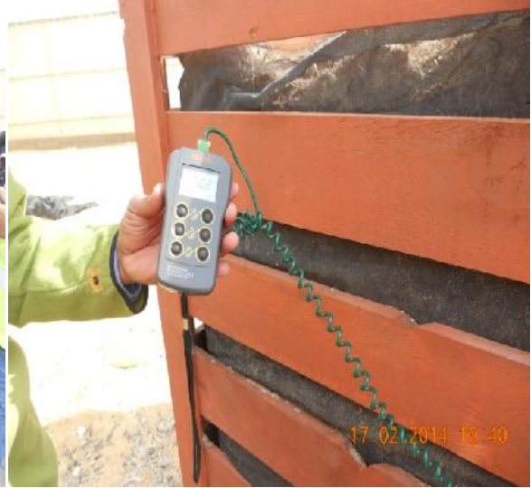
Figure 3.17. Monitoring of compost temperature
