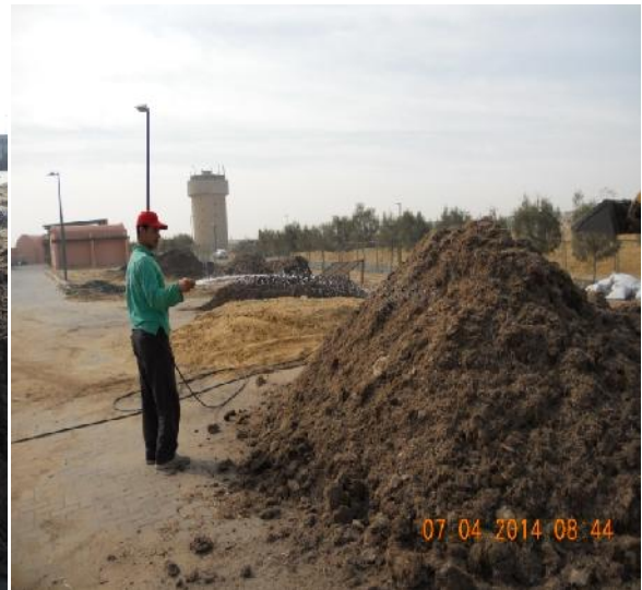
Figure 3.19. Watering of compost windrows
