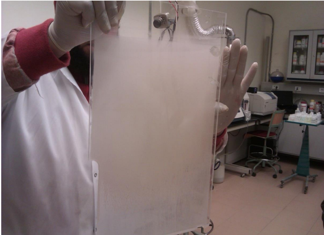
Figure 71: The Lamella with the Accumulated Colloids
