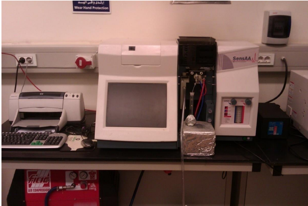
Figure 7: SensAA Atomic Absorption Spectrometer (A.A.S)
