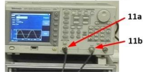
Device# 11: Function generator
