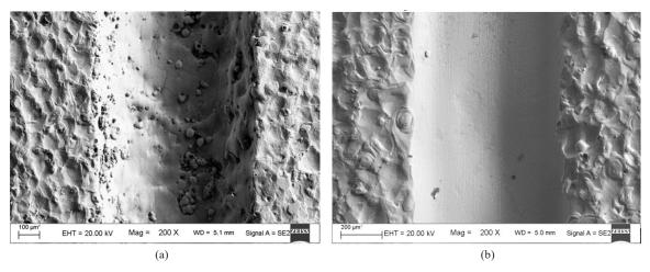
Figure 7. Topography of the microhole surface (a)  $R_a = 1.43 \mu m$ , initial and (b)  $R_a = 0.17 \mu m$ , after abrasive flow finishing (wt. %. of abrasive particle = 45 %).
