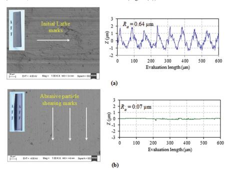
Figure 5. Topography of the tube surface (a) initial (b) after abrasive flow finishing (wt. %. of abrasive particle = 45 %).
