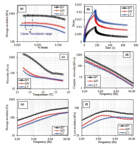
Figure 4. Comparisons of various rheological properties of the high viscous (HV), moderate viscous (MV), low viscous medium (LV) like effect of : (a) % strain on storage modulus (b) time on strain (c) temperature on viscosity (d) frequency on complex viscosity (e) frequency on storage modulus (f) frequency on loss modulus (wt. %. of abrasive particle = 45 %).
