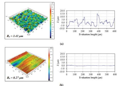
Figure 6. Topography of the microslot surface (a) initial (b) after abrasive flow finishing (wt. %. of abrasive particle = 45 %).
