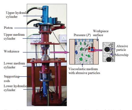
Figure 1. Abrasive flow finishing process set-up with various finishing forces on abrasive particle during the process.
