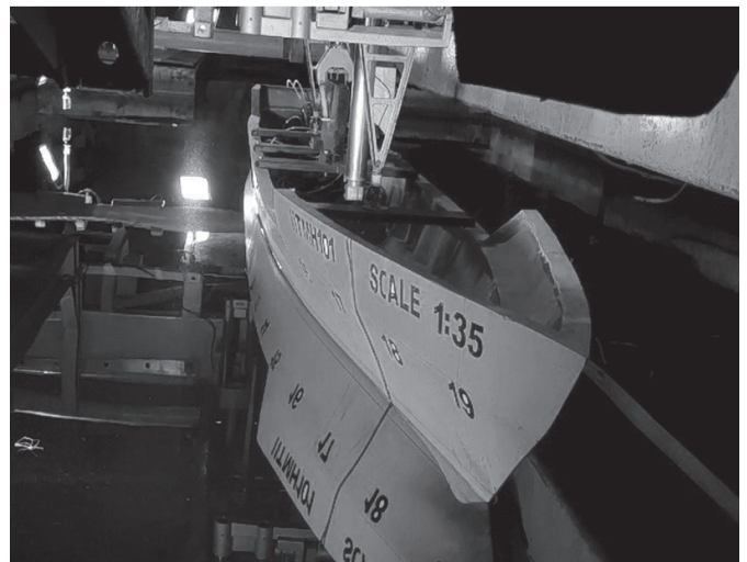
Figure 5. FRP ship model (1:35 Scale).
