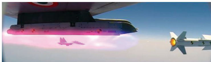
Figure 1. Thermal interference of missile plume with aircraft.
