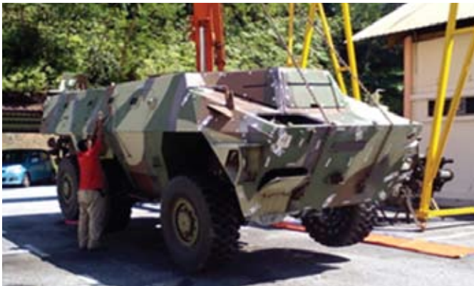
Figure 7. Initiation of the lateral oscillation at the determined vehicle's center line (longitudinal axis).
