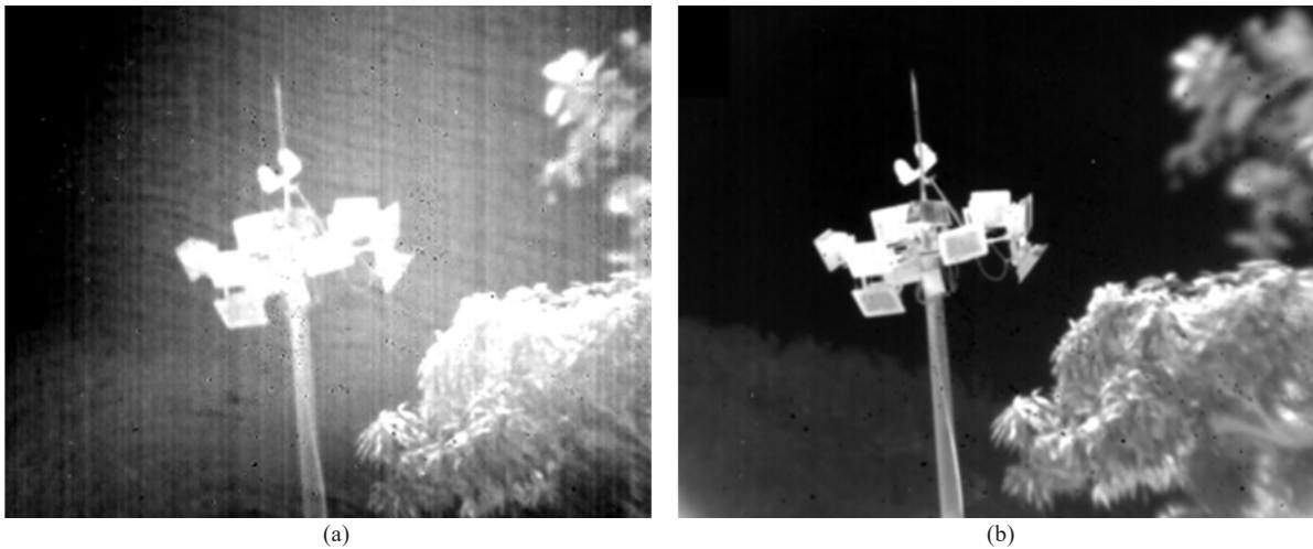
Figure 7. Target 1 image (a) Uncorrected and (b) Non uniformity corrected.
