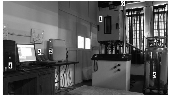
1 Cryo-chamber 2 Controller 3 Operator panel 4 Support computer 5 Liquid nitrogen cylinder 6 Temperature indicator.
