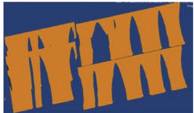
Figure 7. Finite element model and element density after frequency response topology optimisation.
