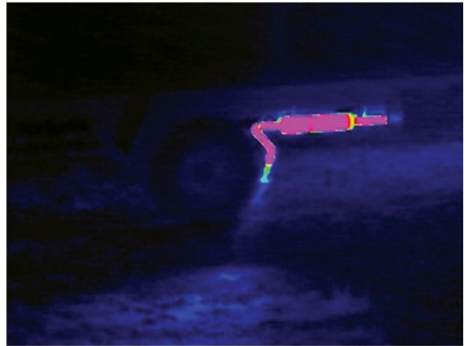
Figure 3. Thermal IR image (3 μm - 5 μm) of truck exhausts in full accelerating engine condition.
