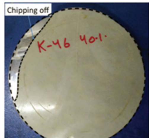
Figure 8. Post-blast visuals of S40 syntactic foam after 5 repeated blast loadings ( P_r \sim 90 \text{ psi} ).
