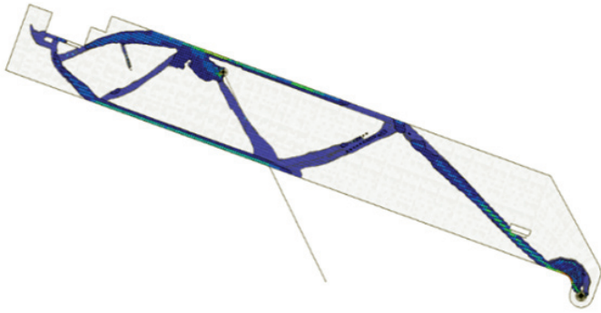
Figure 6. Material density plot for articulation (20°).
