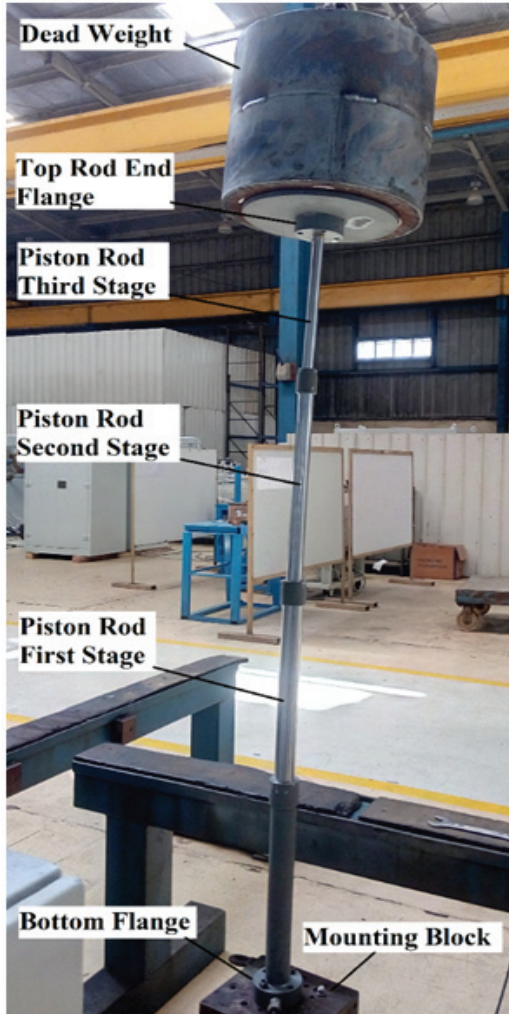
Figure 4. Buckling of three stage nine section fixed free mounting cylinder.
