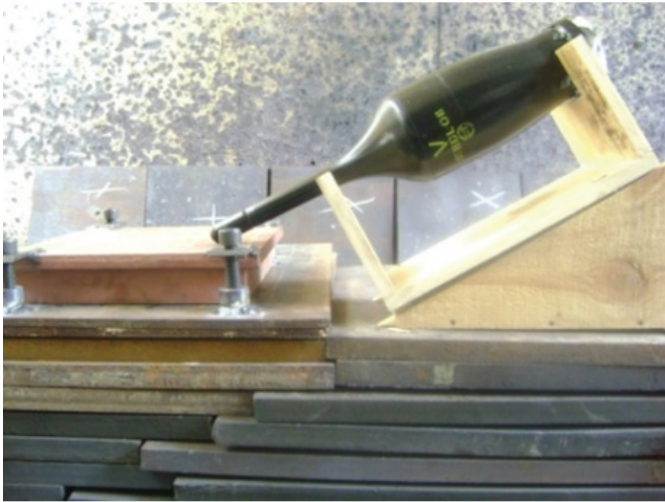
Figure 9. Experimental set up for ballistic evaluation of ERA against shaped charge warhead.
