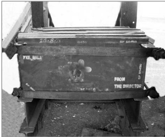
Figure 4. 500 °C tempered steel plates tested against 125 mm FSAPDS ammunition.
