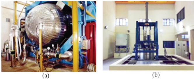
Figure 4. (a) Pressurised acoustic test chamber 14 and (b) Hyperbaric test facility 15 .
