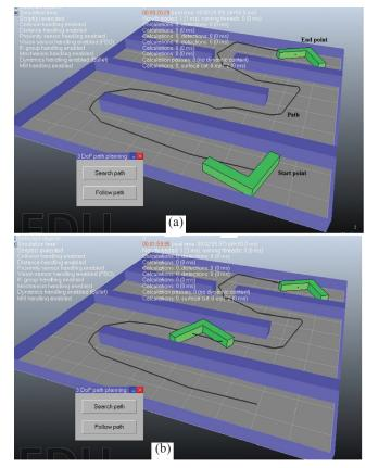
Figure 4. The snapshots of path searching algorithms: (a) Search for a path and (b) Following the searched path.
