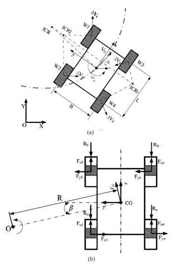
Figure 2. (a) Kinematics diagram for proposed robot and (b) Forces and moments on vehicle.
