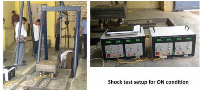
Figure 10. Shock Test on MR mount assembly with controller on and off conditions.
