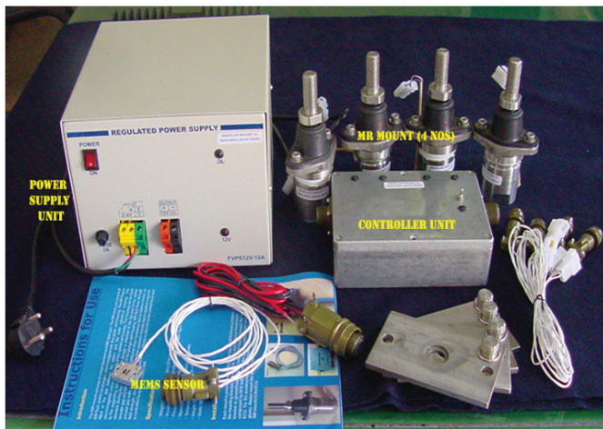
Figure 5. MR mounts with controller unit, MEMS sensor and power supply.
