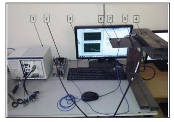
Figure 3. Modal testing of cross-ply Carbon/Epoxy plate specimen of experimental setup.
