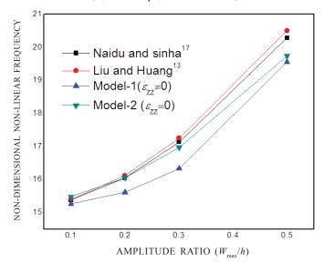
Figure 6. Comparison of nonlinear frequency of a square simply supported symmetric  $(0^{\circ}/90^{\circ})_{s}$  laminated composite plate for (a/b=1, a/h=10).
