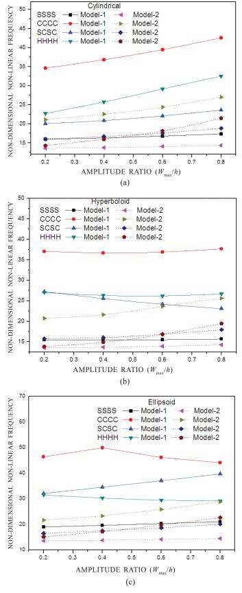
Figure 7. Effect of support conditions on the non-dimensional non-linear frequency parameter of laminated carbon/ epoxy curved panels (a) Cylindrical (b) Hyperboloid (c) Ellipsoid.
