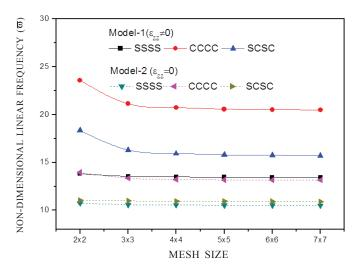
Figure 5. Convergence behaviour of fundamental natural frequency of a simply supported square symmetric cross ply (0°/90°), cylindrical shell panels.
