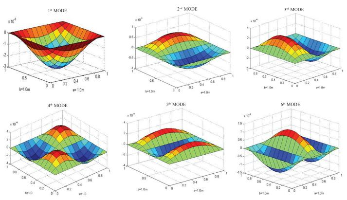
Figure 9. First six mode shapes of a simply supported cross ply laminated carbon/epoxy flat panel.
