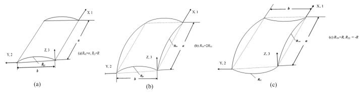
Figure 1. Laminated composite curved panels (a) Cylindrical (b) Ellipsoid (c) Hyperboloid.
