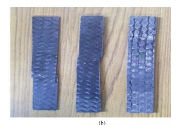
Figure 2. Experimental setup for tensile testing (a) universal testing machine (UTM INSTRON-1195) (b) angle-ply/cross-ply Carbon/ Epoxy specimen.
