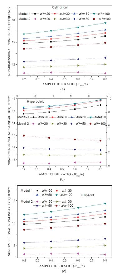
Figure 8. Effect of thickness ratio on the non-dimensional non-linear frequency parameter of laminated carbon/ epoxy curved panels (a) Cylindrical (b) Hyperboloid (c) Ellipsoid.
