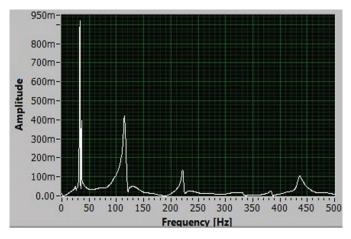
Figure 4. Experimental natural frequency of cross ply Carbon/ Epoxy laminate.
