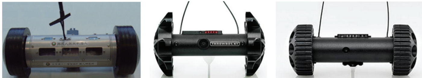
Figure 1. The small scout robots: (a) BIT scout robot, (b) Throwbot XT, and (c) Recon scout IR.
