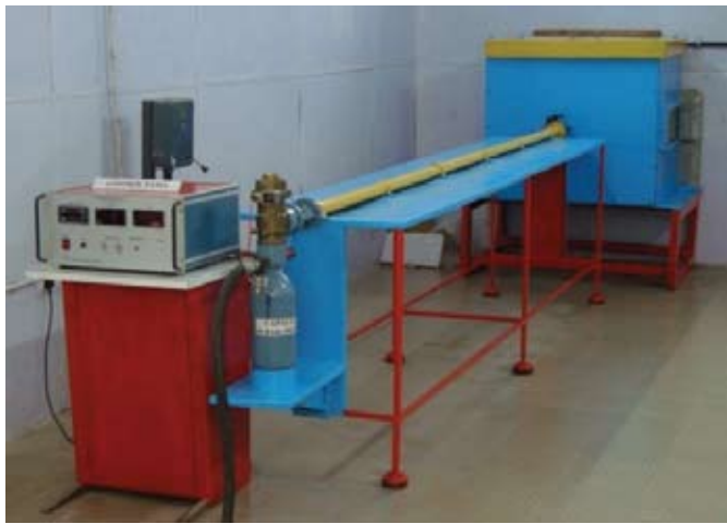
Figure 1. Compressed air gun test setup.
