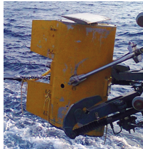
Figure 10. Towed body with depressor.
