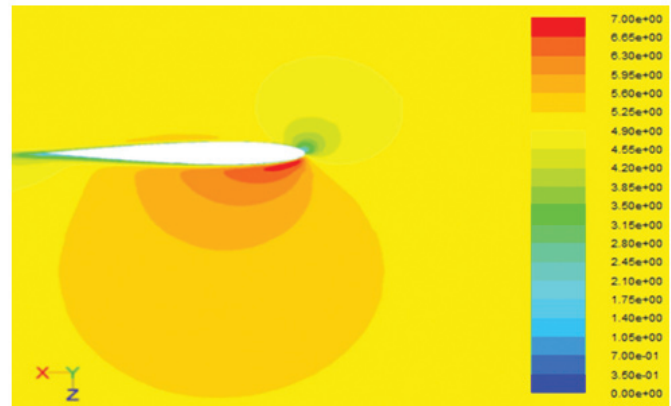
Figure 4. Velocity distribution (m/s) at 10 knots.
