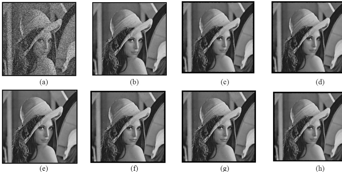
Figure 4. Results of different algorithms for Lena image with 30 per cent noise. (a) Noisy image, (b) ASWM, (c) HEIND, (d) EEP, (e) MDBU (f) CEB, (g) NAFSM, and (h) Proposed algorithm.
