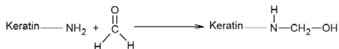
Scheme 3. Formaldehyde absorption by keratin: Available amino groups in keratins chemically interact with formaldehyde
