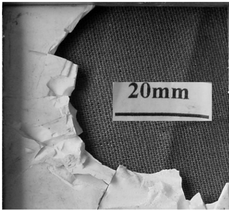
Figure 5. The un-shattered portion of the confined zirconia-toughened alumina (ZTA) after ballistic impact.
