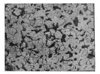
Fig. 5—Pure ferrite grains with inter-connected Porosity after sintering Fe A at 1150°C for 4 hours (X 200) etchant : 1.5% nital solution.
