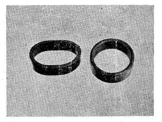
Fig. 2—40 mm dia sintered rings before and after undergoing compression test.
