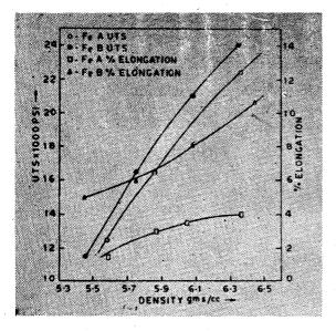
Fig. 3-Tensile properties Vs Density.
