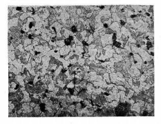
Fig. 7—Ferrite grains with rounded pores and a large region of Fe-Cu phase after sintering Fe-Cu (4% Cu) at 1150°C for 4 hours (X 500) etchant : 1.5% nital solution.
