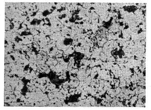
Fig. 6—Ferrite grains with rounded pores after sintering FeBat 1150°C for 4 hours (X 200) etchant: 1.5% nital solution.
