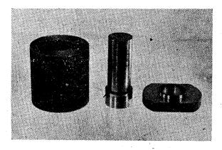
Fig. 1-Die set used for compacting 40 mm I.D. annular rings.
