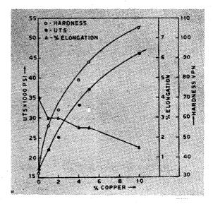
Fig. 4—Sintering Characteristics of  $Fe \ A-Cu$  compositions sintered at 1150°C in liquid phase of copper-
