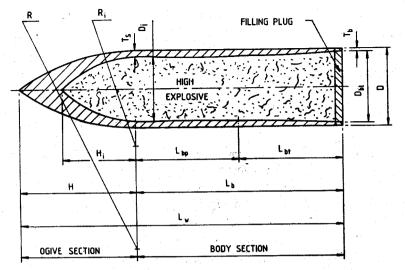
Figure 1. Design elements and parameters of CPES missile-warhead.
