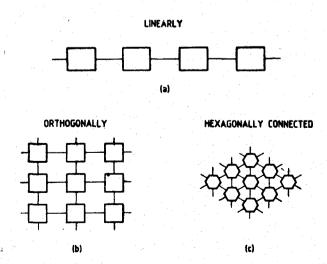
Figure 2. Systolic array configurations.
