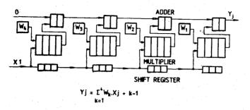
Figure 3. One dimensional convolution array.
