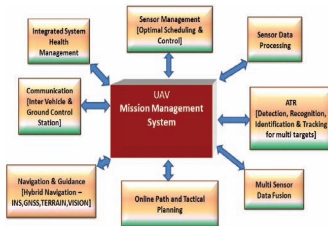
Figure 1. UAV MMS functional components.
