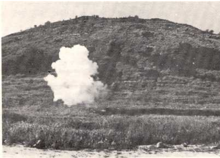
Figure 1. Typical firing of a 40-gm pyro charge. The markings on the poles are 1 m long.
