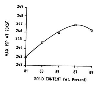
Figure 1. Expected specific impulse for the ISRO polyol propellant.
