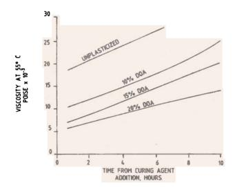
Effect of plasticizer level on the viscosity of 87% loaded IPP 40 ISRO polyol proprilant.
