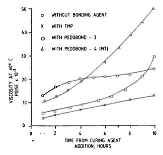
Figure 2. Effect of bonding agent type on viscosity of ISRO polyol propellant.
