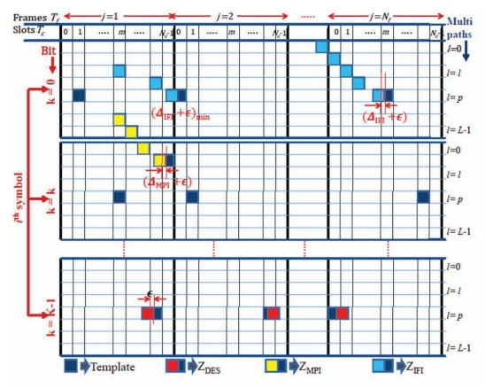
Fig. 4 Pulse correlation between  $p^{\text{th}}$  branch template of  $k^{\text{th}}$  bit with composite received signal.
