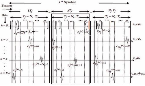
Figure 2. Schematic representation of *M* – ary TH-PSM scheme.
