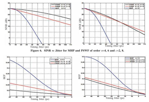
Figure 7. BEP vs Jitter for MHP and PSWF of order n = 4, 6 and c = 2, 8.
