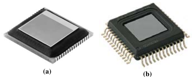
Figure 2. WLP \frac{1}{4} VGA IRFPA onto PCB or in QFP (not at same scale).
