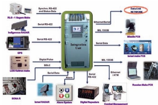
Figure 3. Connectivity of integration unit with various weapons and sensors.
