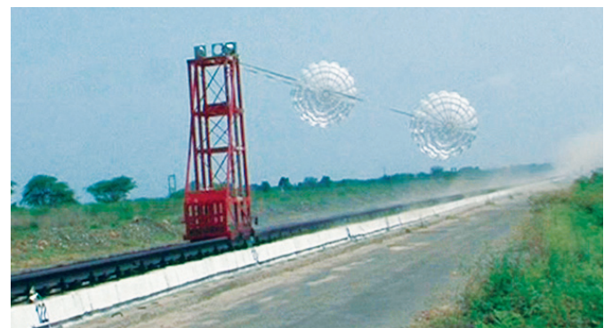
Figure 7. Parachute in deployed condition in RTRS test.
