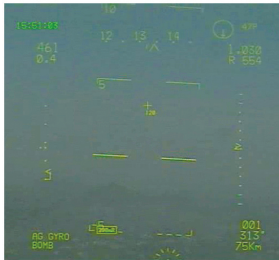
Figure 20. Air-to-ground gyro mode.
