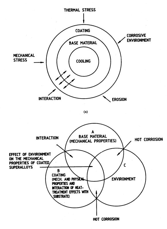
Figure 3. Factors determining effectiveness of coating: (a) substrate and coating, and (b) substrate, coating, and environment
