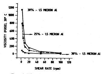
Figure 4. Effect of rpm on viscosity of UDMH-Al gel
