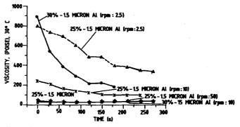
Figure 5. Time dependency and rpm on viscosity of UDMH-Al gel.
