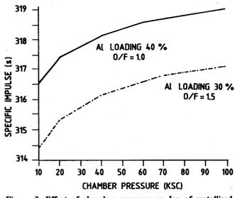
Figure 3. Effect of chamber pressure on Isp of metallised UDMH- $N_2O_4$  propellant.
