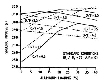
Figure 1. Effect of O/F ratio and Al loading on the performance of UDMH-N<sub>2</sub>O<sub>4</sub> propellant.
