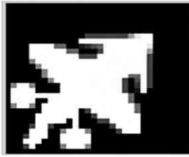
Figure 2. 30x30 pixels image approximating shape of an aircraft. (Fractions ranging from 0.25 to 0.9).
