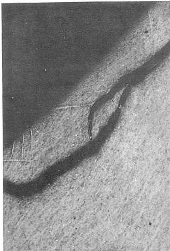
Figure 4. Formation of adiabatic shear bands near the edge of the crater in 20 mm thick steel armour plate at high hardness (520 HV), when impacted by 20 mm diameter steel projectile at normal.
