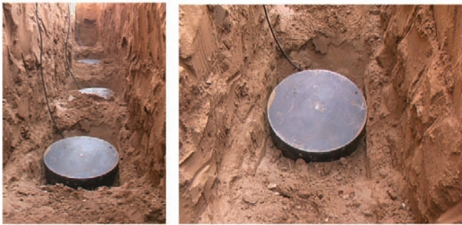
Figure 4. Placement of the pressure transducer.
