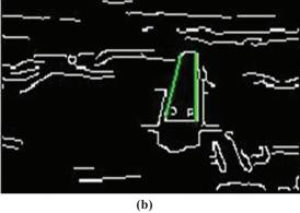
Figure 6. Hough transform on selected search area (a) Runway searched area, and (b) Detected runway edges.
