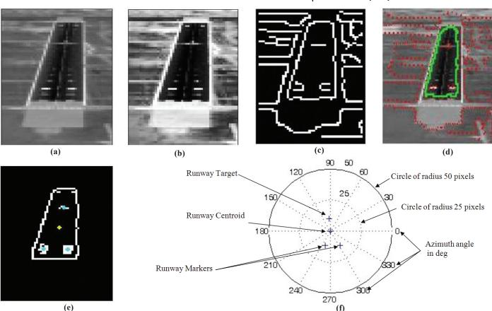
Figure 8. Runway and obstacle detection in normal light condition (a) Cropped image with runway, (b) Enhanced image, (c) Edge detected (binary), (d) Detected edges (labeled), (e) Binary image of runway with markers and target and (f) Location of detected targets and markers w.r.t runway centroid.
