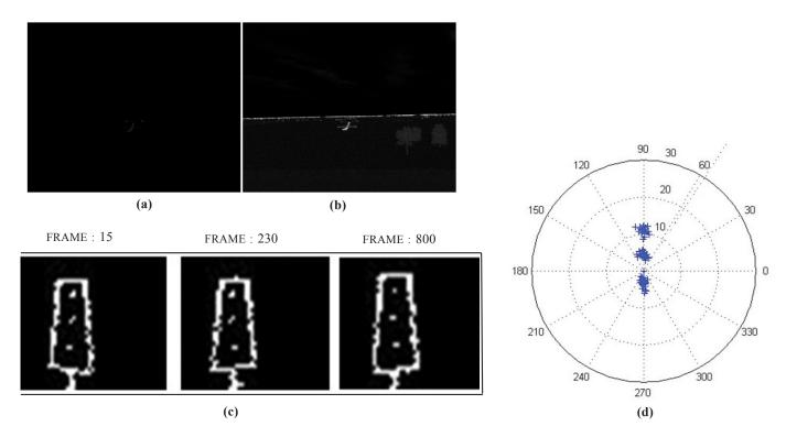
Figure 11. (a) Image from on-board EO camera in fog CAT II visibility in night, (b) Image from on-board MWIR camera in fog CAT II visibility in night, (c) Binary Images of runway with obstacles from MWIR sensor and (d) Location of obstacle with respect to runway centroid.
