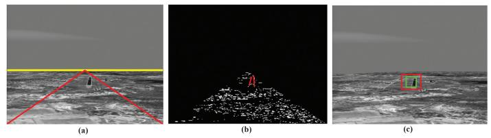
Figure 3. Selection of runway search area by method 1 (a) Initial search area, (b) Runway edge detection and (c) Final search area.
