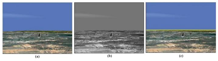
Figure 2. Horizon detection (a) Original image, (b) Gray level image and (c) Image with Horizon line.
