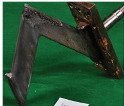
Figure 9. Photograph of one of the stage-II struts (strut-2L) after the test.
