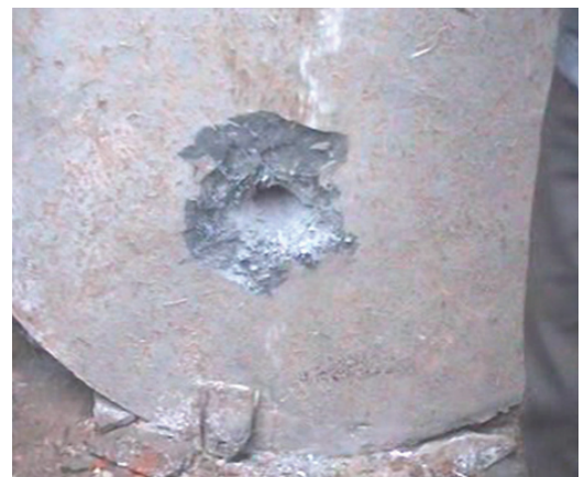
Figure 3. Typical features of SFRPC targets after penetration (the first group).
