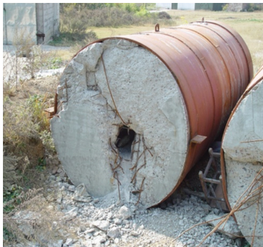
Figure 4. Target No. O-1 after penetration.
